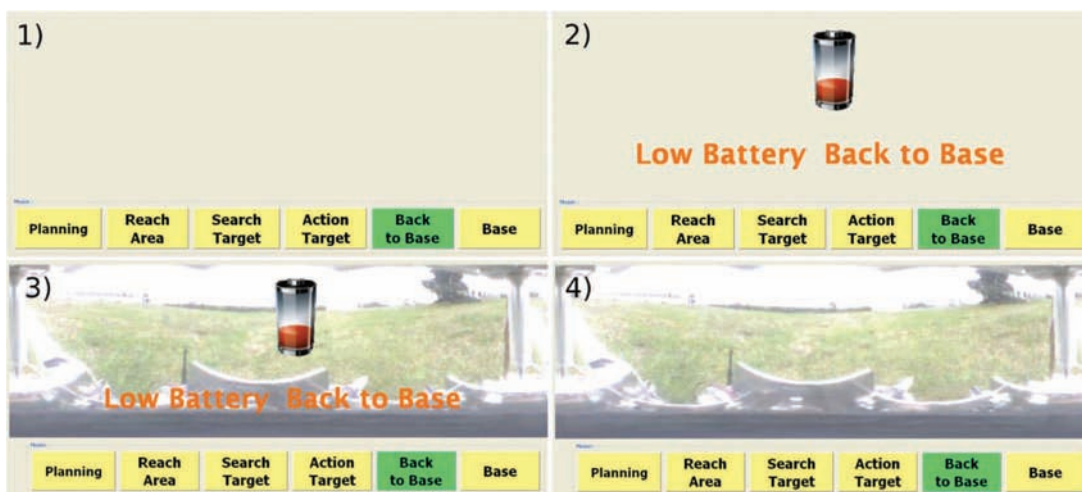
Figure 3. These four panels respectively represent the four steps of the cognitive countermeasure dedicated to disengage the human operator’s attention focus from the panoramic video and to enhance his or her situation awareness. Top left panel, Step 1: The panoramic video was removed for 1 s. Top right panel, Step 2: The relevant information to understand the behavior of the robot was placed in the human operator visual field for 3 s. Bottom left panel, Step 3: The video panoramic screen reappeared with the relevant information superimposed on it for 3 more seconds. Bottom right panel, Step 4: End of the cognitive countermeasure. Note that the robot was stopped while the cognitive countermeasure was triggered.
