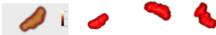
FIGURE 5.3. Left: Grey level template estimated from the 3D murine dendrite spine excrescences. Binary volume (second image) is created by thresholding the previous continuous image. (Third and fourth images) Two spine excrescences templates estimated from the mixture deformable template model.
