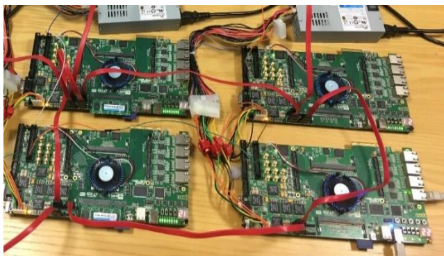
Fig. 5. A 4 FPGA AstroByte platform with SATA connections
