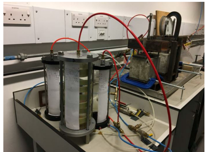
Figure 3 : Extended water penetration test setup
