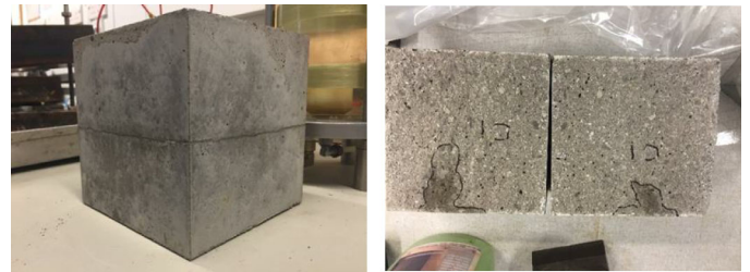
Figure 2: Jointed sample before and after the water penetration test
