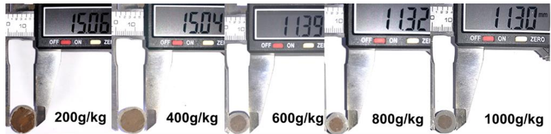
Figure 6. Cross-section of CS-LWA green body with different amounts of coating materials.
