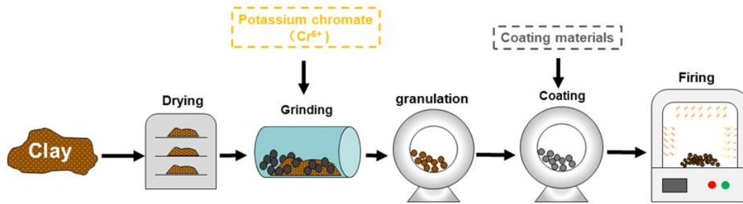
Figure 2. The experiment process of CS-LWA preparation
