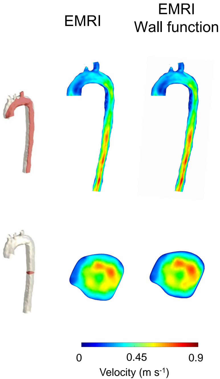
Figure 5.20: Velocity maps of the aorta ( t=0.2348 s) computed with EMRI and EMRI with Wall function. Sagittal cutting plane (top row) and transversal cross section (bottom row). The locations of cutting planes are shown on the left panel.
