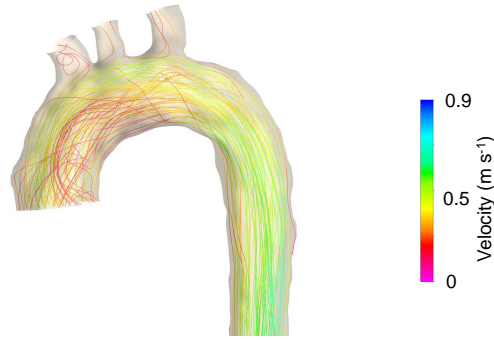
Figure 1.11: Visualization of the flow patterns of a patient specific CFD model of the aortic arch.
