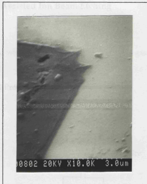
Fig. 5.8 SEM photograph of a corner of a masked area
