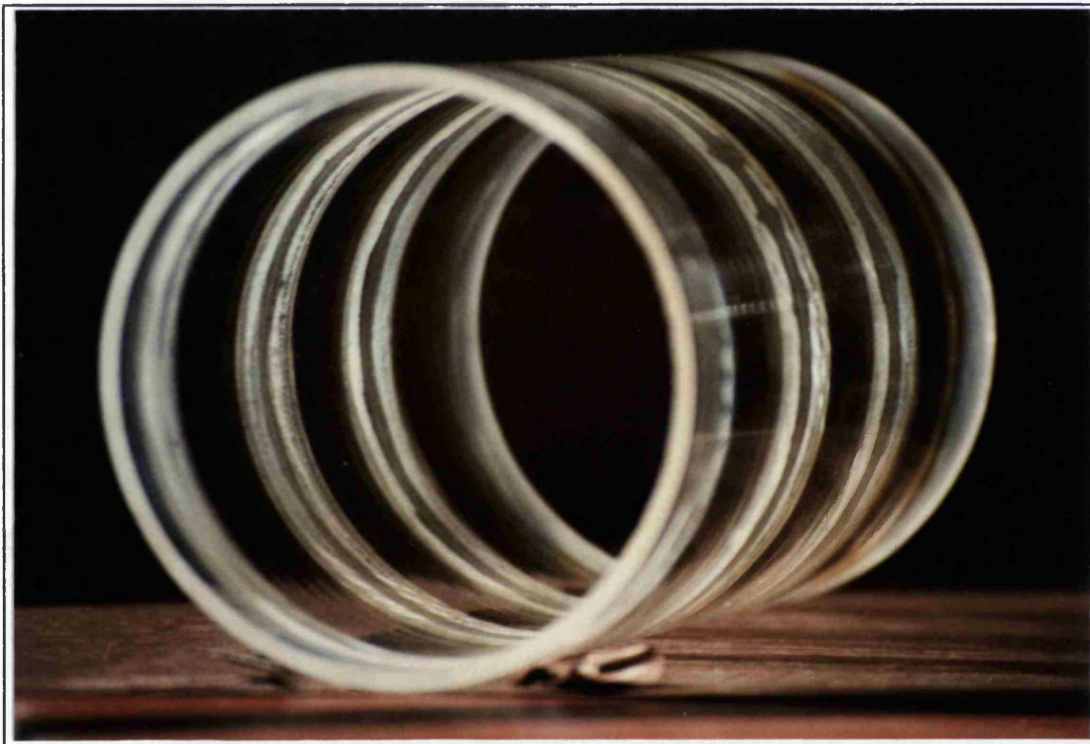
Fig. 5.14 Photograph of silica liner showing erosion
