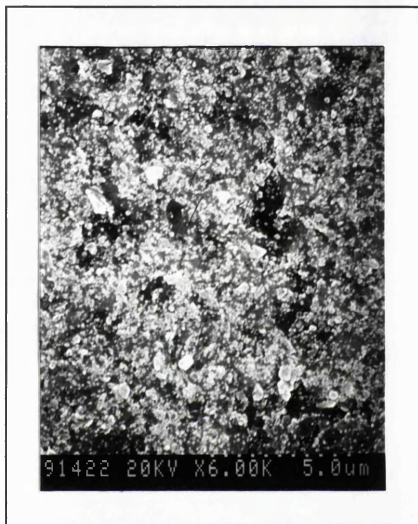
Fig. 9.6 SEM photograph of sample (v), grown with rf power 250W for 17 hours
