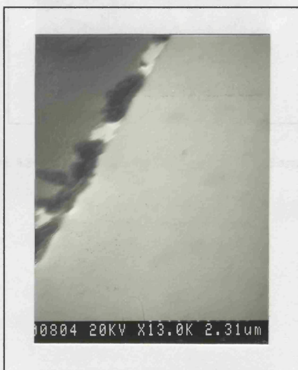
Fig. 5.7 SEM photograph of the RIBE etched surface
