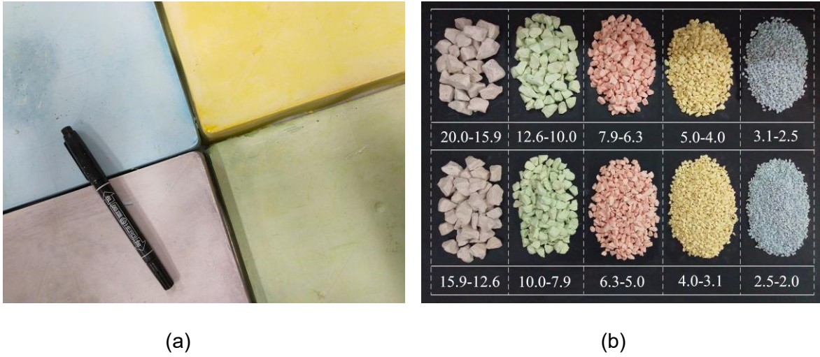
Fig. 1. (a) Manufactured dyed gypsum boards; (b) dyed gypsum particles (DGPs) (parent particles)
