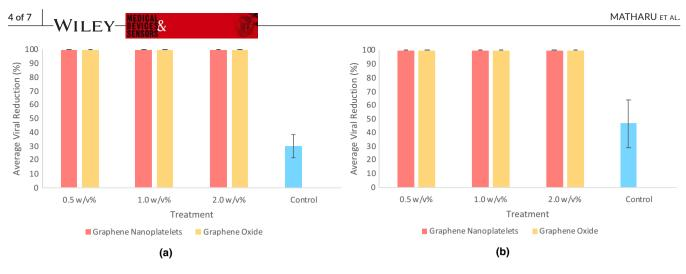
**FIGURE 2** Antiviral activity of graphene nanoplatelets and graphene oxide nanosheets at 0.5, 1.0 and 2.0 w/v% against T4 bacteriophage after (a) 3 hr and (b) 24 hr of exposure. Control samples were exposed to no treatments. Error bars represent standard deviation (n = 3)
