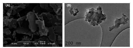
**FIGURE 1** (a) Scanning electron micrograph of graphene oxide nanosheets and (b) transmission electron micrograph of graphene nanoplatelets
