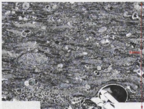
Figure 4.24: A slightly lighter area within the dark sediment from rock slab 11. In the bottom right bivalve remains can be seen. The scale of the image is 600\mu\text{m} from top to bottom. Taken on the Southampton BSEM by Dr. Richard Pearce.
