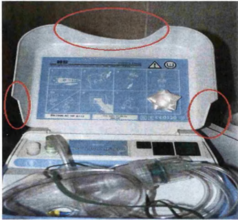
Figure 4.5: Compressor with a broken lid
