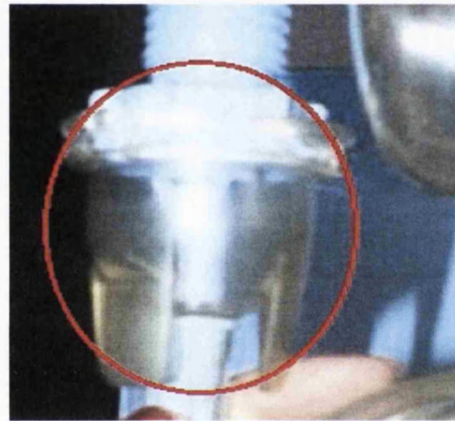
Figure 4.8: Discoloured nebuliser chamber
