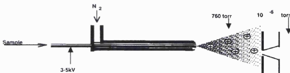
Figure 6.3: Pneumatically assisted electrospray ionization. Adapted from (Brewer and Henion, 1998)
