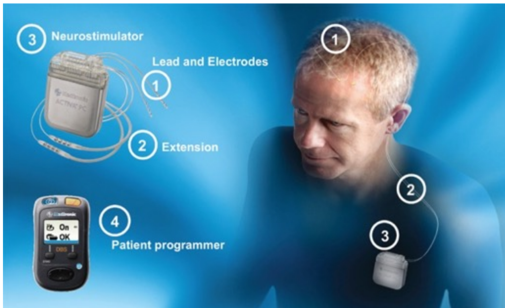
Figure 1.2. Deep brain stimulation system (Medtronic Activa PC™ device).
