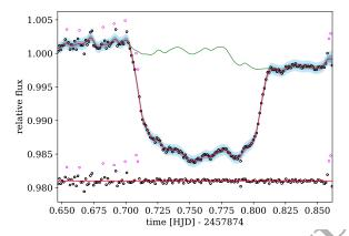
**Figure 2.** White light curve of WASP-103b obtained with the 600B grism. The red line shows the best fit model with blue shading indicating plus/minus two standard deviations. The green line shows the systematics model derived from the GP fit. Residuals are indicated below the light curve. We clip any points over  $4\,\sigma$  from the fit, but preserve them for the common-mode correction (shown in magenta, see Section 3.1).
