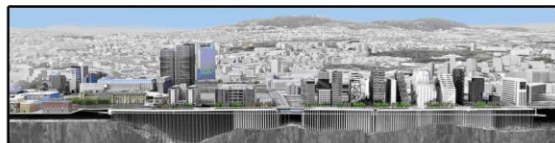
Figure 1: Dronning Eufemias gate, Oslo. The picture integrates the support structure of the road, clearly visualizing the three-dimensionality of infrastructure.
