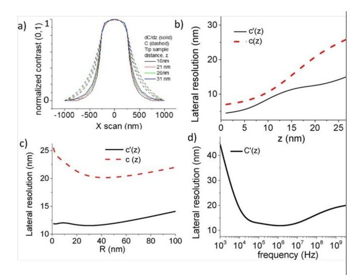
Experimental comparison of EFM lateral resolution and electrical contrast at different frequencies.
