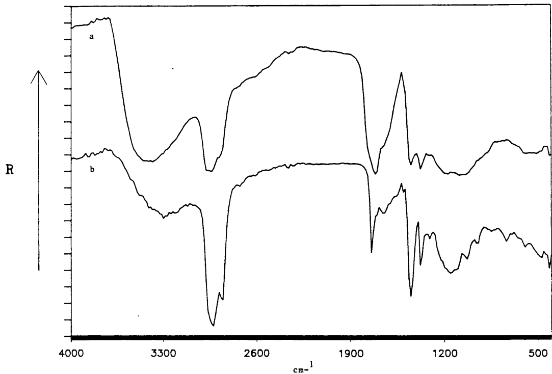
Figure 13.1 Diffuse reflectance FT-IR spectra of samples from (a) a gutta percha inkwell (PHS1) and (b) a vulcanite Vesta box (PHS14) from the Plastics Historical Society collection.
