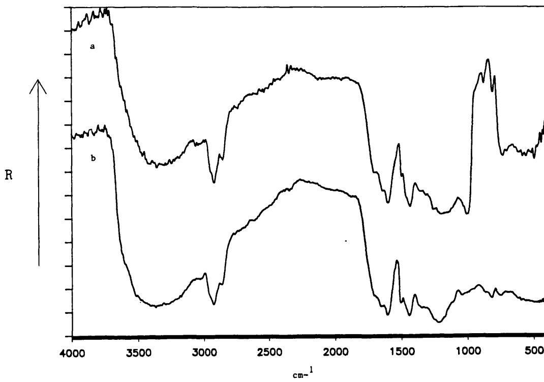
Figure 6.7 Diffuse reflectance FT-IR spectra of (a) black bead (DM3) found in cemetery at Verulamium, St. Albans (V7532 #127) (gsva0413) and (b) jet from Whitby Museum (GS16) (gsva0517).
