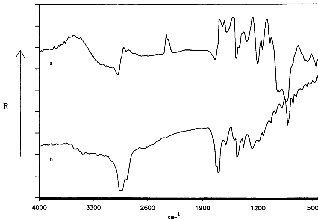
Figure 3.4 Diffuse reflectance FT-IR spectra of (a) softwood pitch (RW1 Pix liquida) (gsva0015) and (b) softwood pitch mixed with KBr powder (RW1) (gsva0615).
