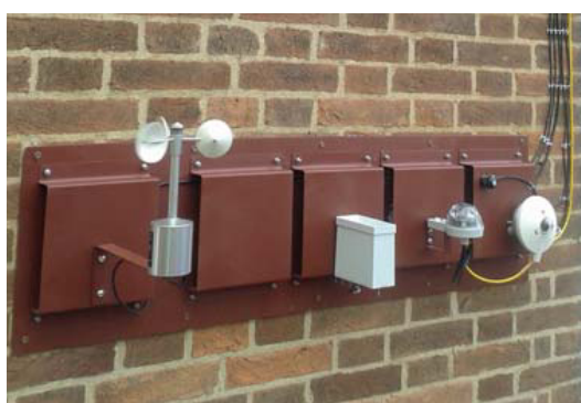
Fig. 3. Climate monitoring equipment. L to R: Vector A100R anemometer, Pronamic Rain-o-Matic tipping bucket rain gauge; Hydreon RG-11 optical rain gauge; Apogee SP110 silicon-cell pyranometer; Kipp and Zonen CMP3 pyranometer.
