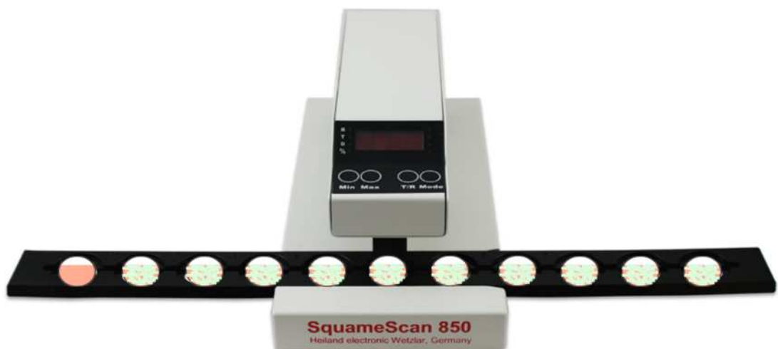
Figure 2.2. The SquameScan 850 measures the absorbance % on D-Squame tapes after tape stripping (Modified picture from clinicalandderm.com).
