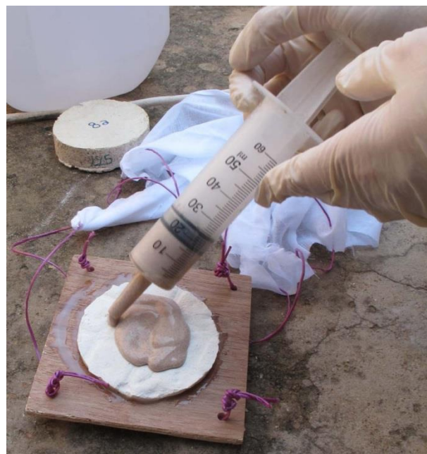
Fig.4: 'Sandwich' test preparation for grouts MG (coarse-araish plaster delamination) (©The Courtauld Institute of Art, 2016)
