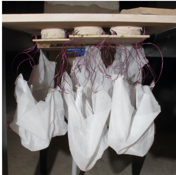
Fig.3: 'Sandwich' test for grouts G (stone-coarse plaster delamination) (©The Courtauld Institute of Art, 2016)
