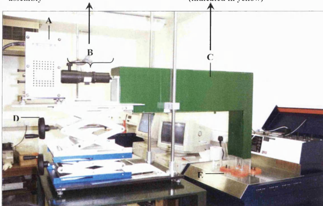
Figure 2.1a: (a): IR filter; (b): shutter; (c): cooling system; (d): focusing lens assembly
