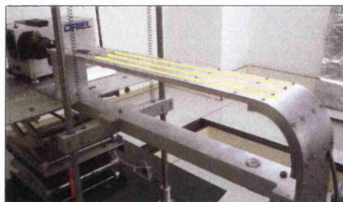
Figure 2.1b: Optical cables contained within stainless steel light guide (indicated in yellow)
