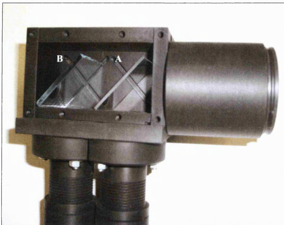
Figure 2.25: Open view of light box; A: polka-dot mirror; B: first surface mirror
