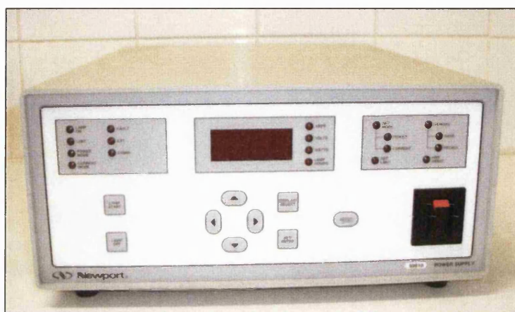
Figure 2.17: Digital Power Supply used to provide constant power to the lamp
