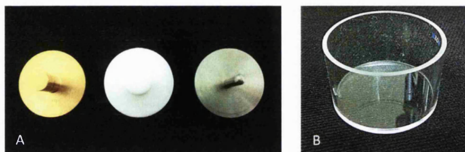
Figure 3.2 NIR transfectance analysis: (A) three types of the reflector discs; gold, plastic, and silver; (B) quartz reflectance cell.
