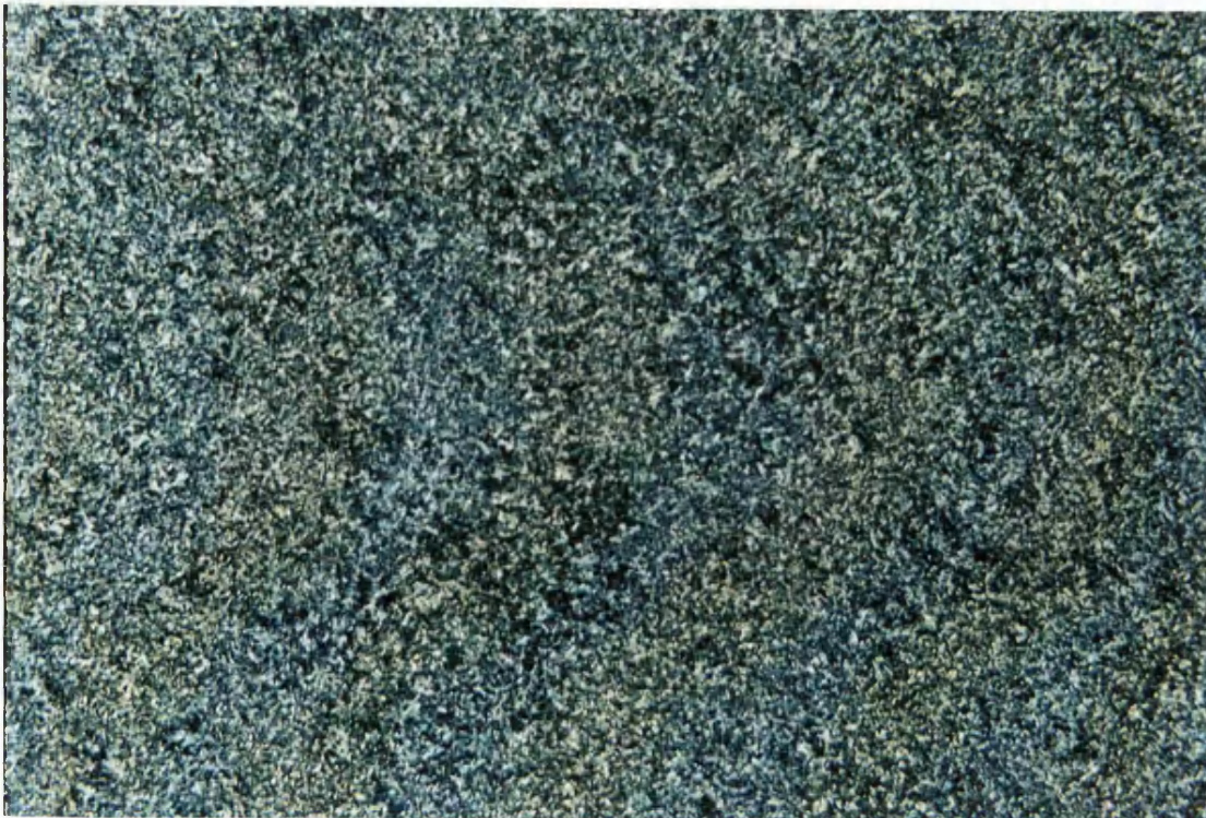
Plate 7.8: Pure G50/13 aged for 7 days at 37°C under crossed-polars 1:110
