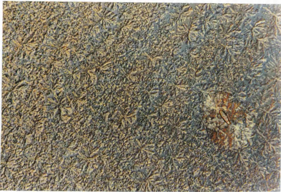
Plate 3.15: 10% paracetamol in G50/13 at 25°C during cooling
