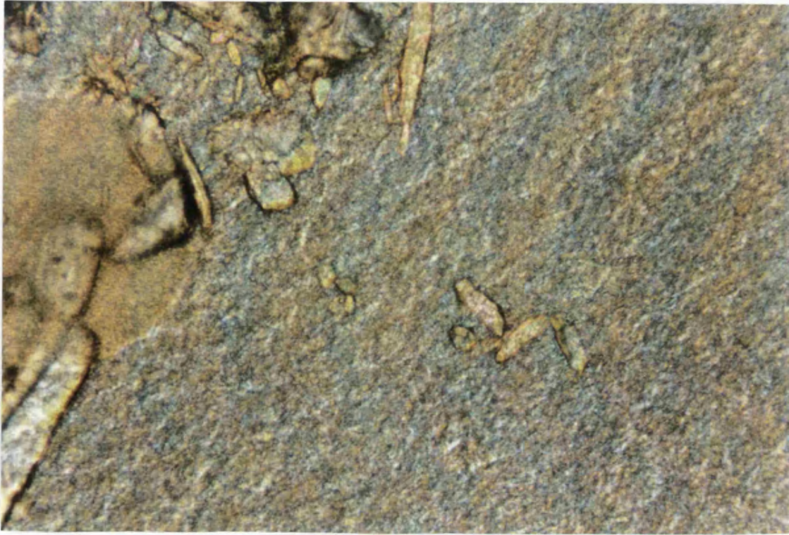
Plate 3.11: 5% paracetamol in G50/13 at 25°C after 10 minutes holding during cooling
