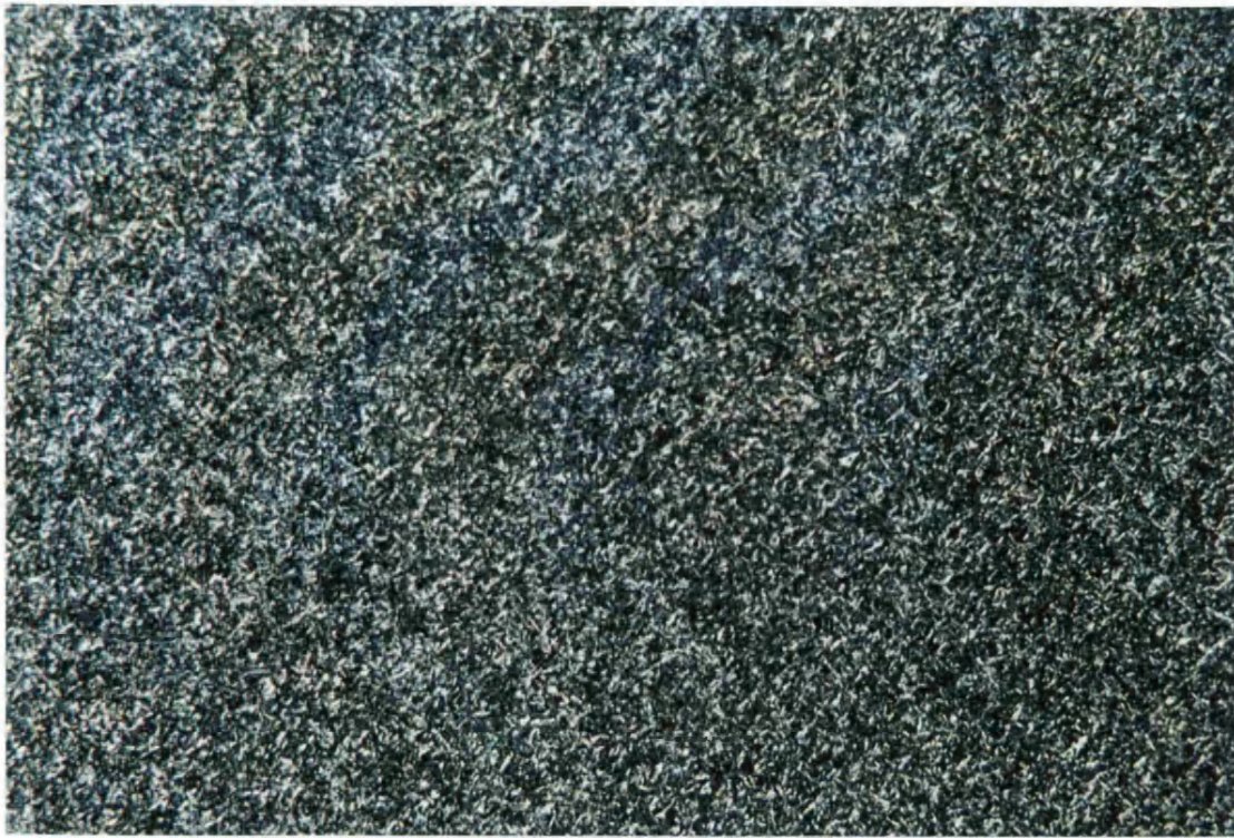
Plate 7.5: Pure G50/13 aged for 7 days at 20°C under crossed-polars 1:110
