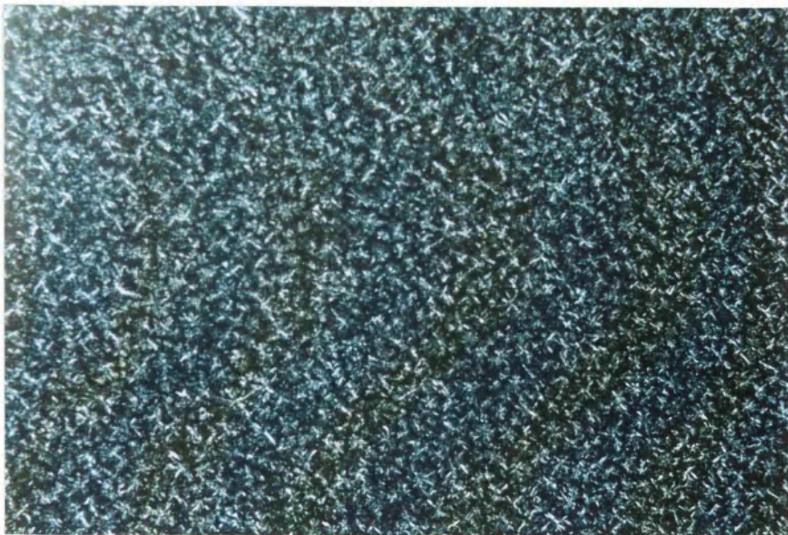
Plate 7.6: Pure G50/13 aged for 7 days at 20°C under crossed-polars at 44°C 1:110
