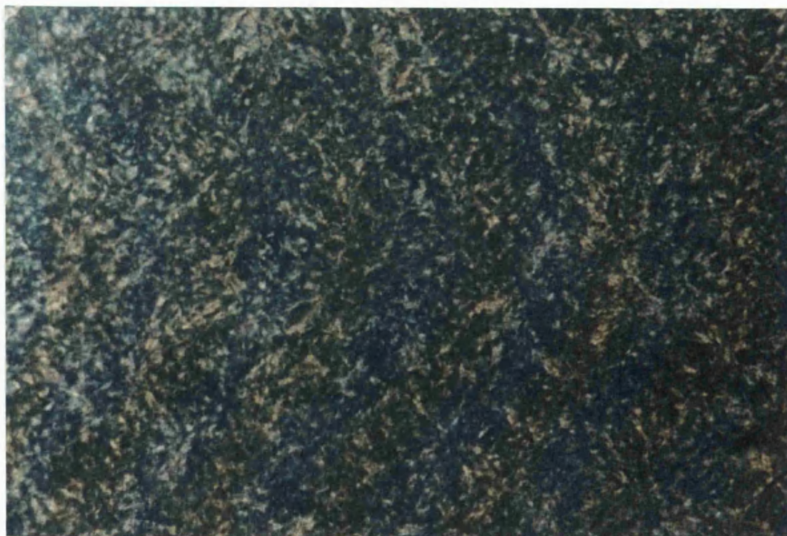
Plate 7.14: 10% paracetamol in G50/13 aged for 7 days at 37°C under crossed-polars 1:440
