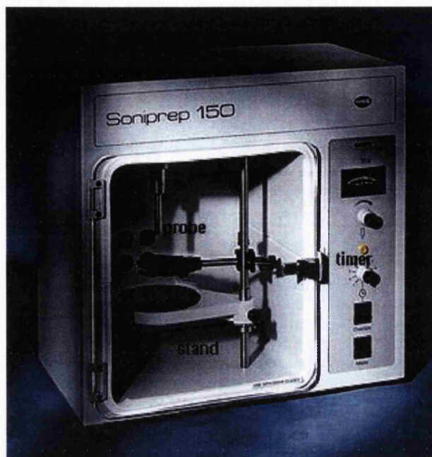
Figure 2.1: Sonicator (Sanyo MSE Soniprep 150, Sanyo Gallempkamp PLC, Leicester, UK) used to prepare PLGA-PEI nanoparticles.
