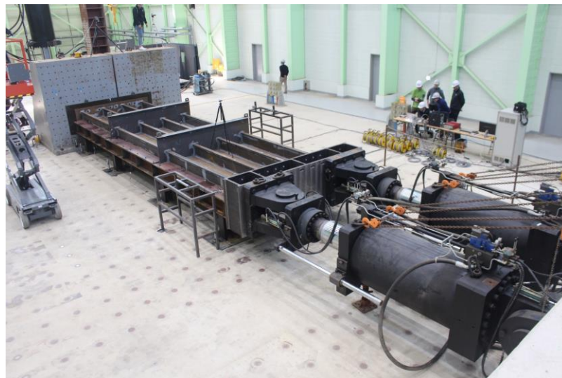
Figure 15. The test set-up of the structure with jigs at the KOSORI test site.
