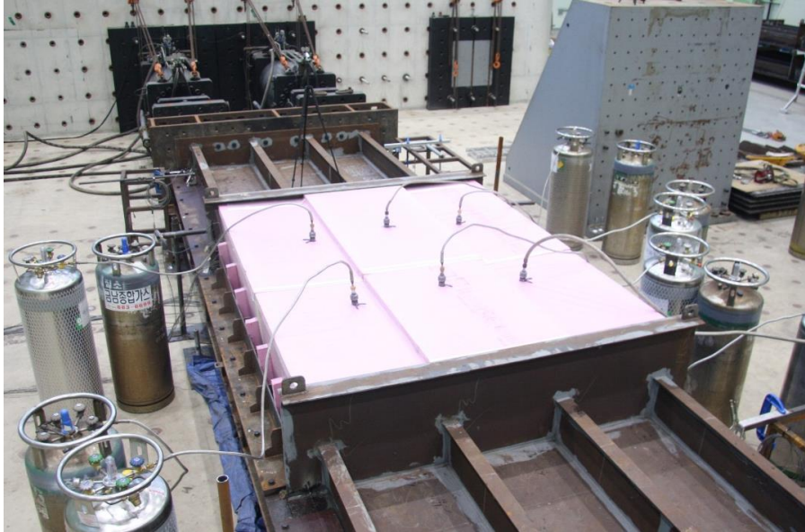
Figure 16. Pouring of nitrogen gas at the central bay of the tested structure.
