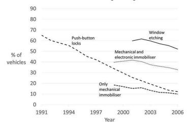
**Figure 2.** Decreasing vehicle security devices.
