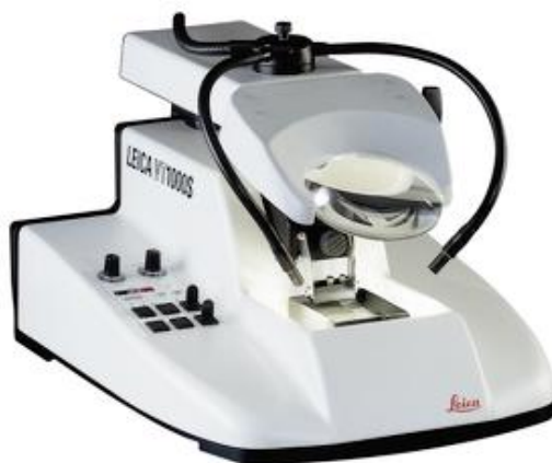
Figure 2.2 VT 1000 Vibrating Blade Microtome used to perform brain slices 300 \mu m thick. The image to the right is a close-up of the stage where the slices are produced (Leicabiosystems.com).
