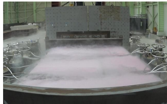
(b) Injection of liquefied nitrogen gas
