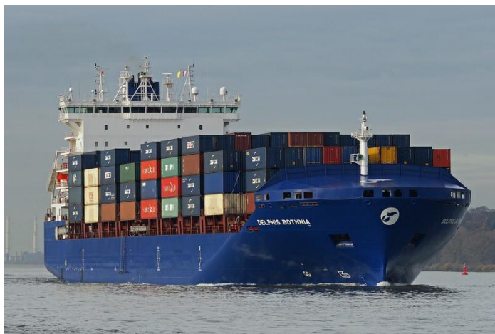
Figure 7. The reference vessel used in this study, a 1,900 TEU containership built by Hanjin Heavy Industries, Busan, South Korea.
