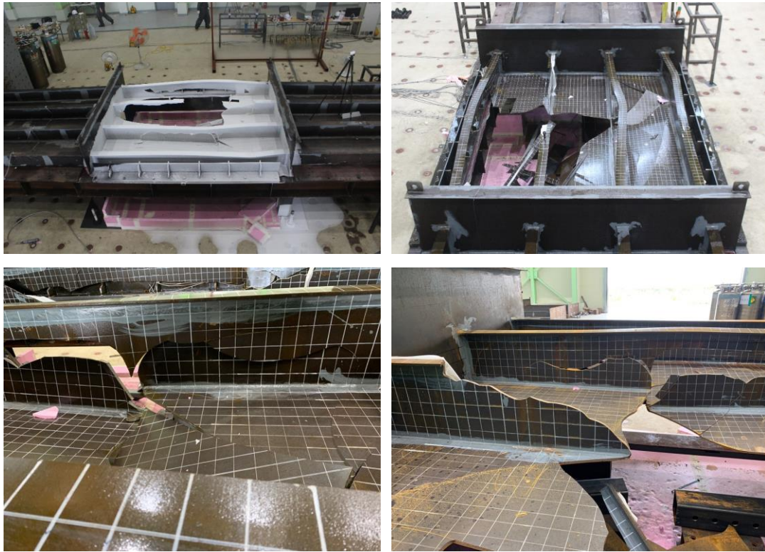
Figure 30. Brittle fracture of the test structure at cryogenic condition.
