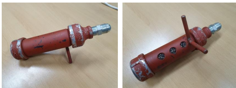
Figure 24. Specially designed nozzle to spray liquefied nitrogen gas into the central bay of the test structure.
