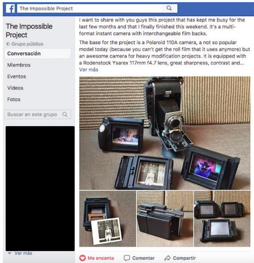
(Fig. 32) Screenshot of a Polaroid Roll Film Camera Adapted To Instant Format posted on The Impossible Project Facebook
