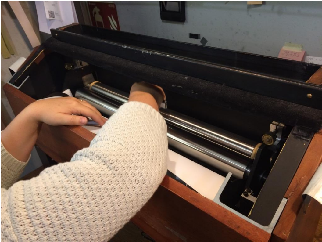
(Fig. 35) Elisa Explaining how to Calibrate the 20x24 Processors Rollers
