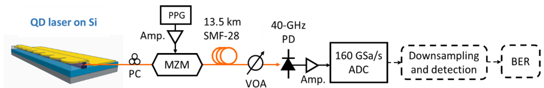
Figure 3.7 Setup of data transmission experiment. PC: polarisation controller; Amp: RF amplifier; PPG: pseudorandom pattern generator; SMF-28: standard single-mode fibre; PD: photodetector; ADC: analogue-to-digital converter; BER: bit-error rate.
