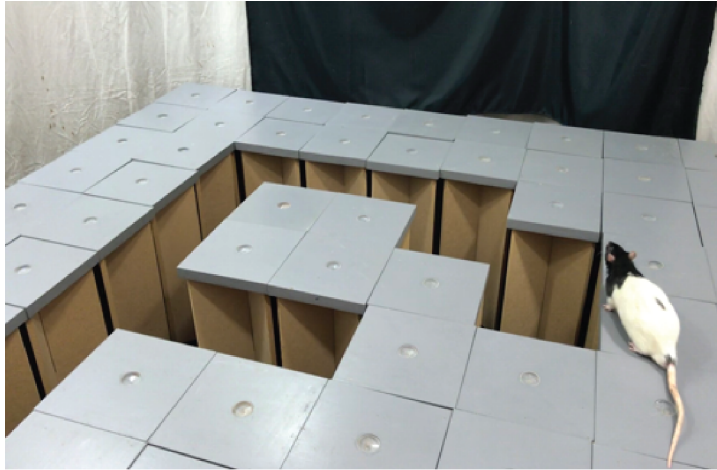
Figure 2.2: The maze environment used for the rat experiment. The environment consists of 100 removable maze modules with a black curtain over one of the surrounding edges to provide a single extra-maze cue. Reward can be dispensed at the goal module by filling the well with chocolate milk via polymeric tubing beneath the maze.
