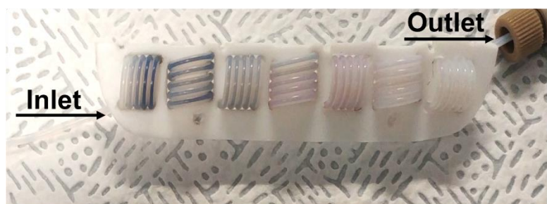
Figure D-3 Picture of the PTFE-made mixing stage used for reactant mixing ( HAuCl_4 and H_3Ct:Na_3Ct ) after leaving the mixer filled in with the reacting solution overnight. Particle deposition (fouling) appeared on the tube walls. Arrows indicate the inlet and the outlet of the reacting stream.
