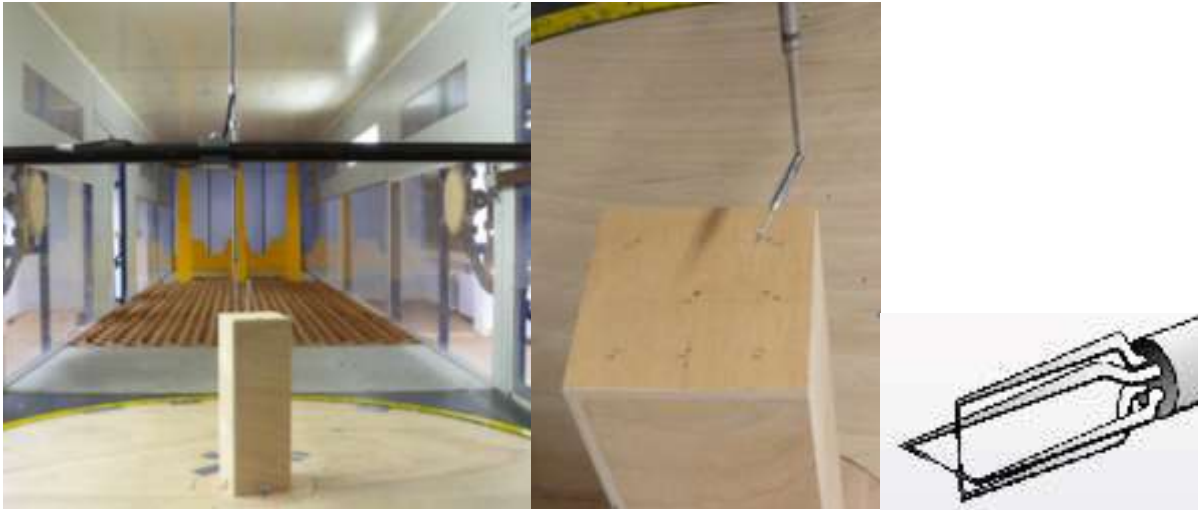
Figure 4.5. Photo of the wind tunnel with the model mounted on a turning table
