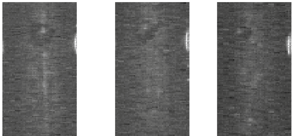
Fig. 3 Images taken with the apparatus of Fig. 1, cropped to remove some of the light that had diffracted around the outer pipe wall. The images are at 10^\circ intervals, with the sample rotated clockwise from left to right
