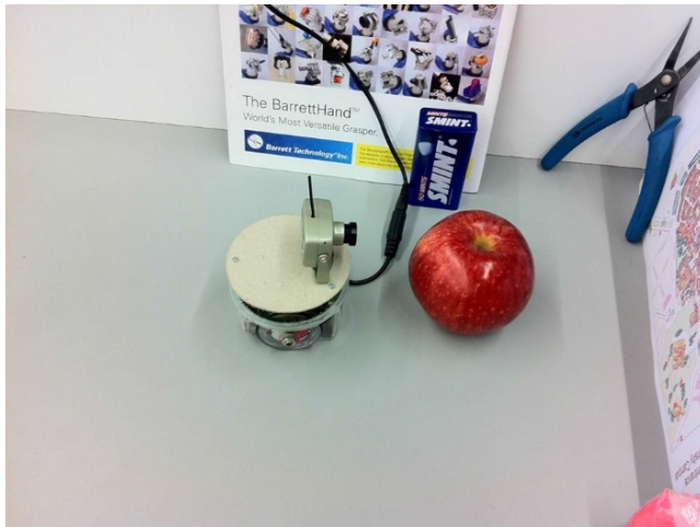
Figure 4: One of the E-Puck’s intentions is satisfied by perception of the color red. If that intention were active, this would be a rewarding state for the robot. If the other intention were active, this would not be rewarding. When the reward signal is positive, all colors detected in the image are gradually associated with the CoS for that intention. It is essential for the robot to see different background colors. Of course, if one never sees a teacup apart from its saucer, one will never understand they are two separate objects.
