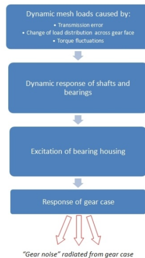
Figure 3: Noise transmission path
