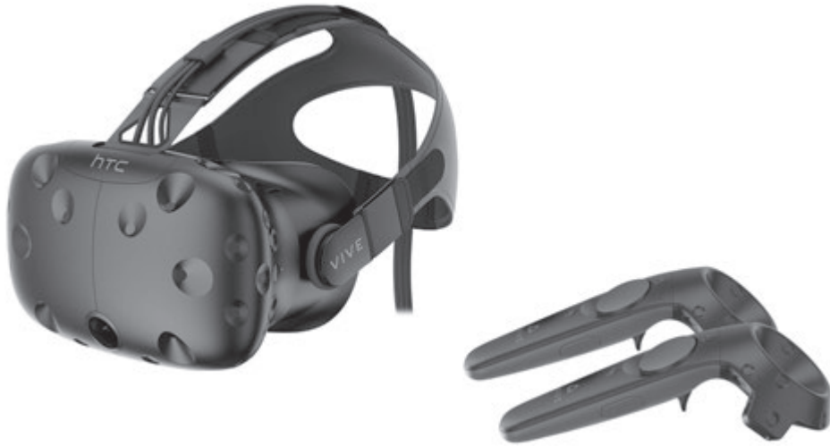
Figure 1 Example of a virtual reality head-mounted display (left) and controllers (right). This is the HTC VIVE system (HTC Corporation, New Taipei City, Taiwan).
