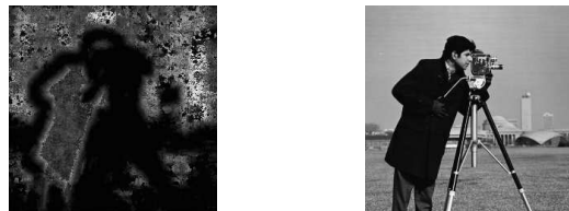
Fig. 5: Patch-sizes selected for each pixel in the cameraman image reconstructed at \sigma = 25 . Dark pixels indicate small patches, and brighter pixels larger patches (Left). The clean image (Right).
