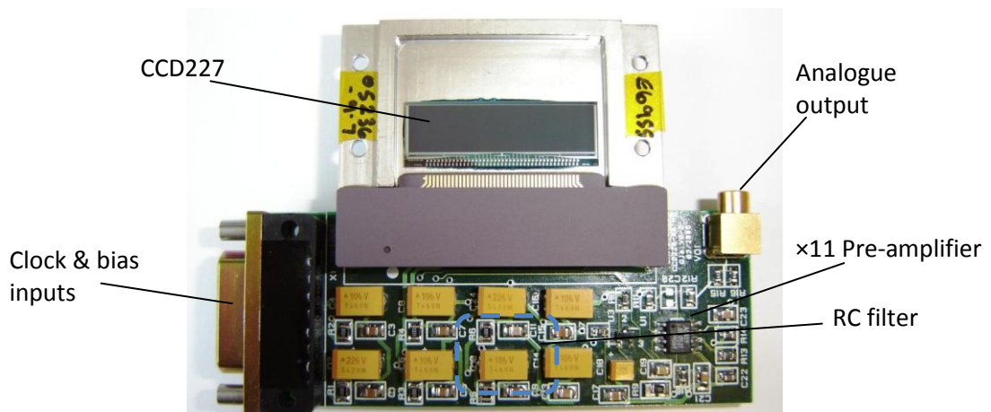
Figure 4.17 e2v CCD227 and bias filtering 'headboard' developed under this work
