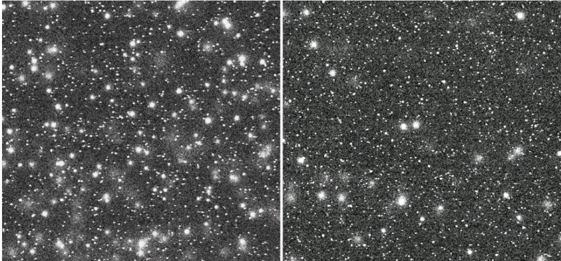
Figure 6.14 X-ray event patterns observed by CCD247 at V_{ss} = 0 V (left) and V_{ss} = -100 V (right)
