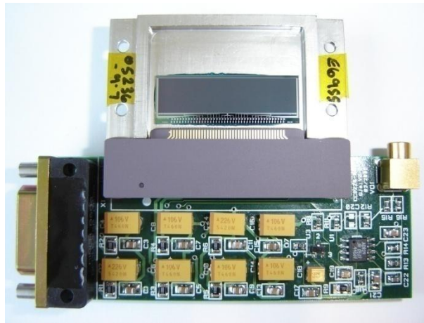
Figure 5.20 High resistivity p-channel CCD (CCD227) and headboard
