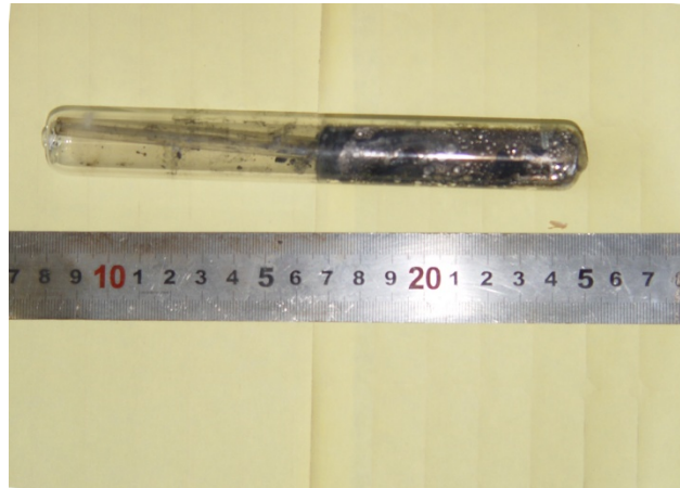
Fig.1 The quartz glass tube before heating at 873 K
