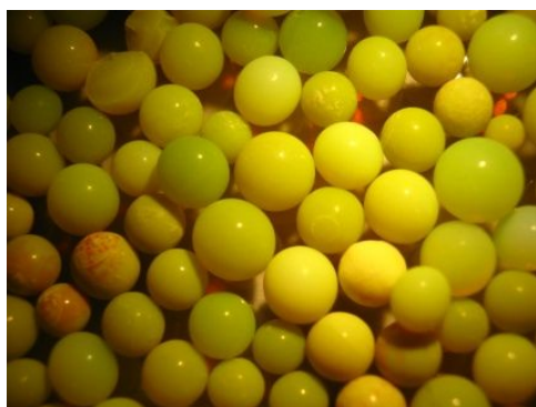
Fig. 5 An example of a SILP containing chlorocuprate(II) ionic liquid impregnated porous 4 mm diameter silica spheres.
