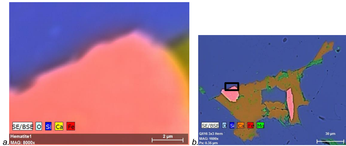
Fig. 8 SEM-EDX analysis of top-left hematite inclusion and its surrounding dielectric gangue matrix. The exact location across the large sample area is highlighted by the black square in Fig. 8b. a. collects the contribution from the different chemical elements, detailed in c.
