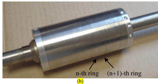
Fig. 15. Photos of the wound stator (a) and rotor (b) assembly
