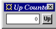
Figure 1. A sample Fudgets program. intDispF is an integer text fudget that uses a text box for interaction, mapstateF keeps a counter, and buttonF is a button fudget. >==< chains fudgets from right to left, placing them next to one another in the GUI.
