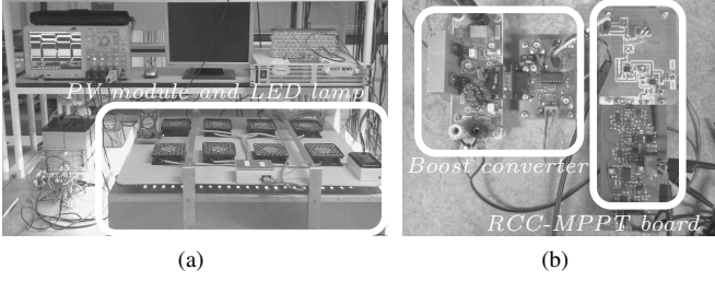
Fig. 8. Fig.8a: PV module and LED solar emulator and Fig.8b: boost converter and sliding-mode RCC-MPPT analog control board.
