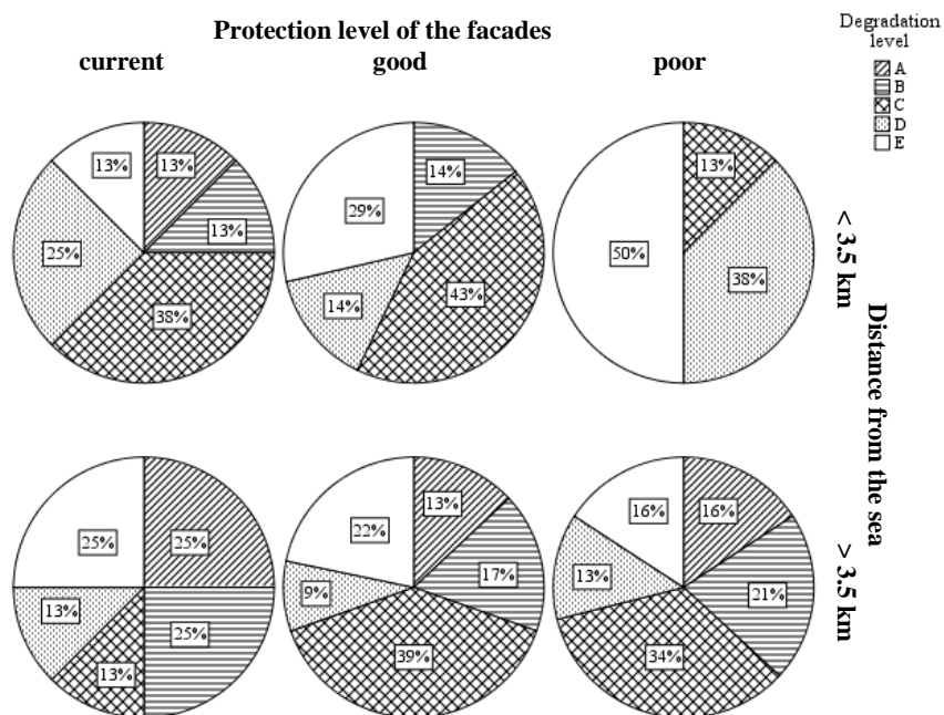
Figure 13 - Analysis of the different degradation levels according to the distance from the sea and the protection level of the facades
