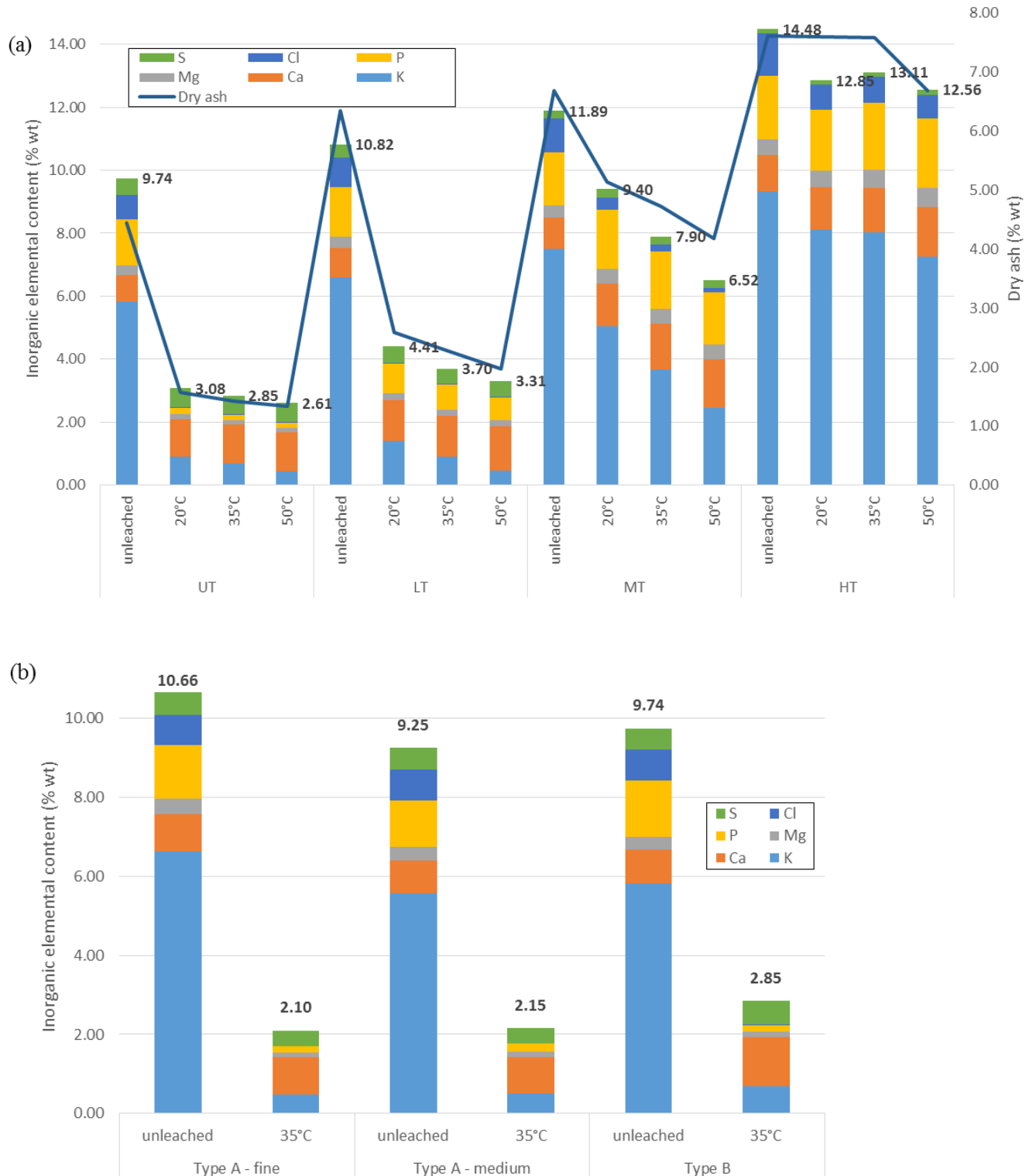
Fig. 3. Total inorganic content from XRF for leached and unleached (a) untorrefied and torrefied type B and (b) untorrefied type A and type B.
