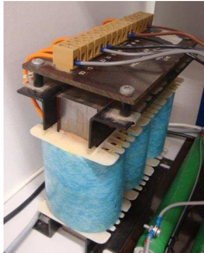
Fig. 7.8 Input filter inductor.
