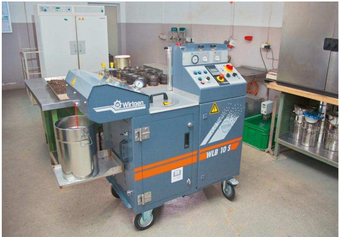
Figure 2-8: A Wirtgen Foam Bitumen Rig
