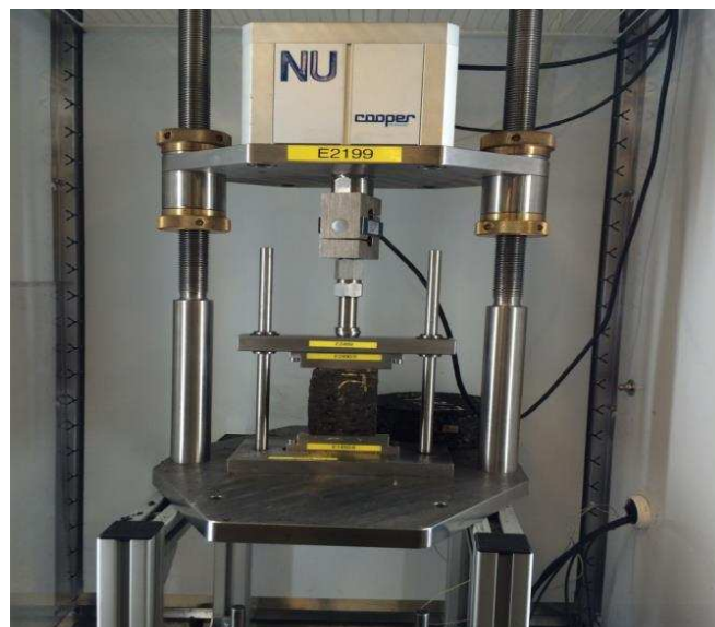
Figure 5-3: Test set up for Indirect Tensile Fatigue Test (ITFT)
