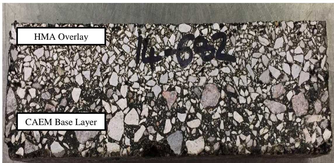
Figure 6-6: A Typical Beam for WTT
