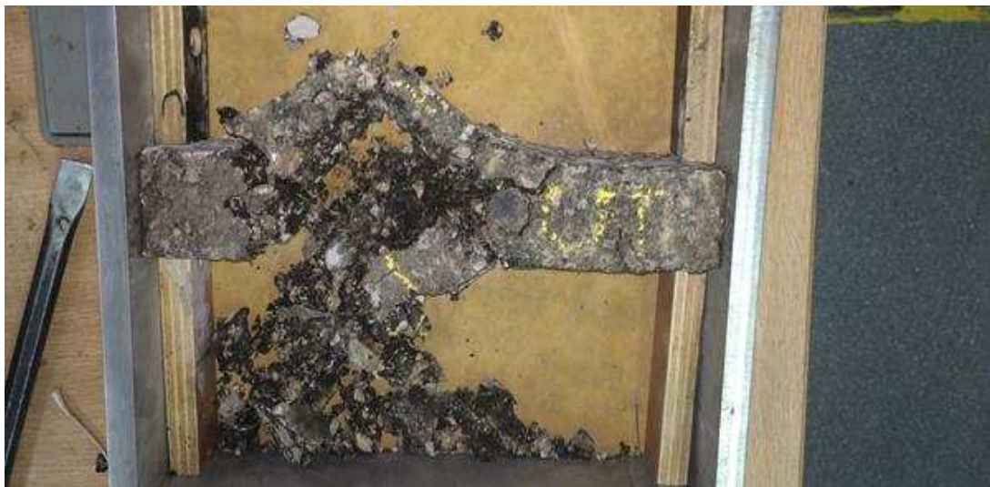
Figure 6-8: Total Failure of the 80mm thick CAEM Base Layer
