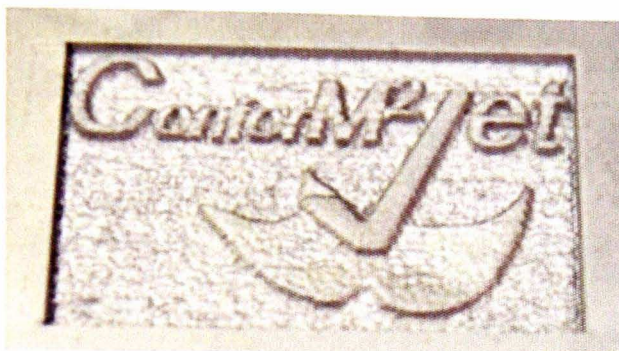
Figure 8-7: ConforM 2 -Jet logo milled in Ti-6Al-4V based on the traverse speeds computed by the developed mathematical model [40].
